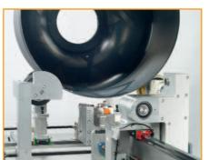
PlasmaJet® with pendulum nozzle Special machine construction The photos on the left demonstrate some possible uses for plasma pretreatment with customer-specific components. In this case, it refers to the processing of round hollow bodies for the aerospace industry.
