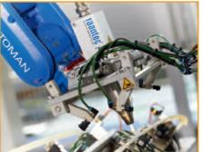
Due to the selection of the outlet nozzles, hard to access part geometries such as, e.g. complex contours or three-dimensional bodies can be treated.
